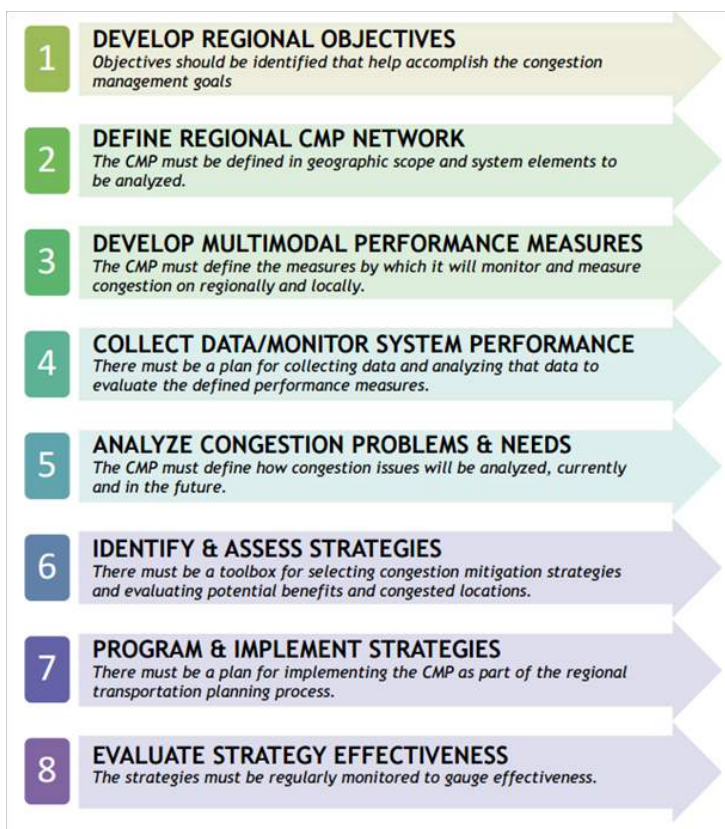
Figure 8-2: Federal Eight-Step Congestion Management Process
